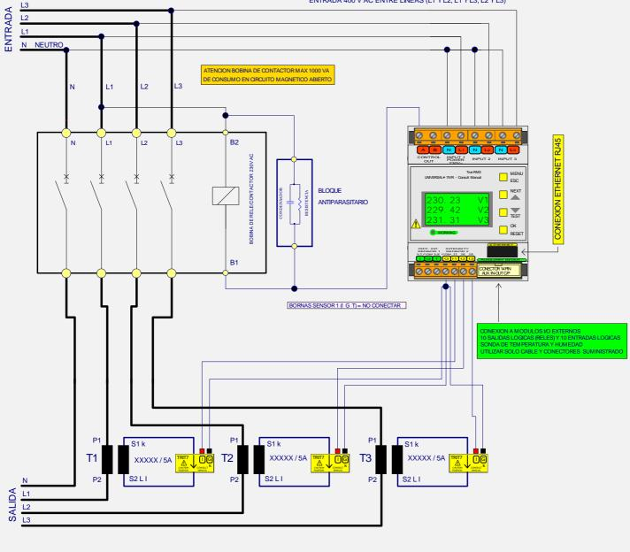
ENTRADA 230 V AC ENTRE NEUTRO Y LINEAS (L1, L2, L3) ENTRADA 400 V AC ENTRE LINEAS (L1 Y L2, L1 Y L3, L2 Y L3)
