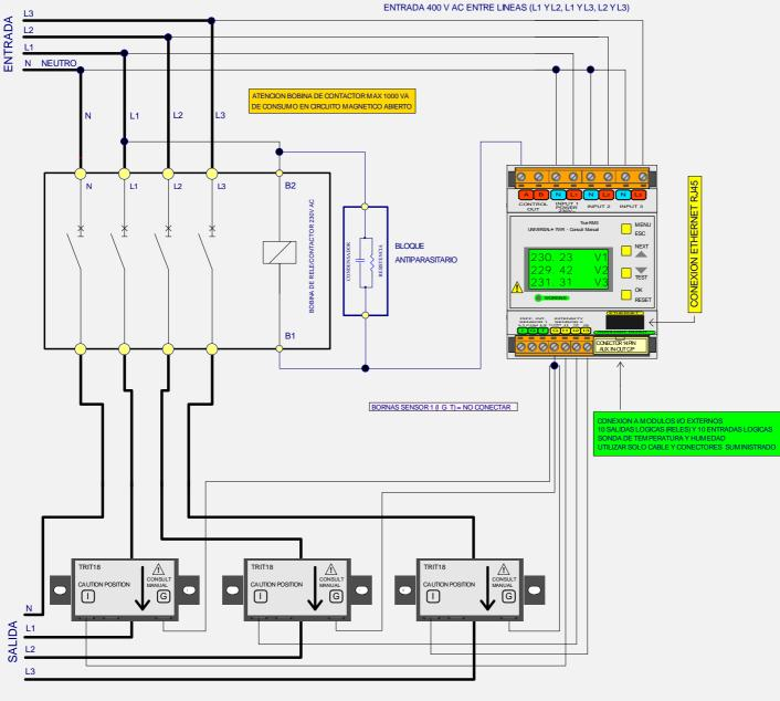
ENTRADA 230 V AC ENTRE NEUTRO Y LINEAS (L1, L2, L3) ENTRADA 400 V AC ENTRE LINEAS (L1 Y L2, L1 Y L3, L2 Y L3)
